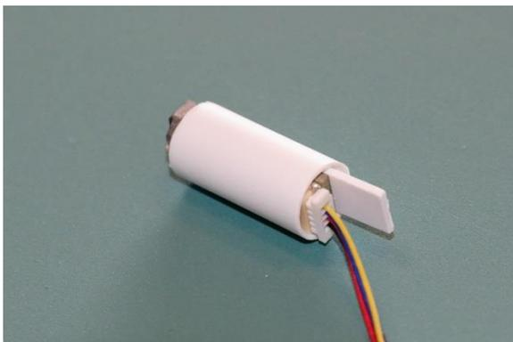
To secure the detector within the tube, slide a 3/4" long Evergreen styrene 0.040" x 0.250" strip behind the detector. The fit will be tight. If the 0.040" strip can't be inserted, a 0.030" thick strip should work.
