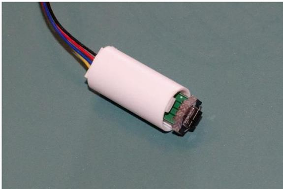
Pushing the detector up from the bottom of the tube will provide room for careful application of epoxy to the top of the styrene strips that contact the top "hat" of the detector. After the epoxy is applied, push the detector onto the top of the holder so that the "hat" sits down on the tube and styrene strips.
