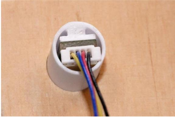
When the styrene strip is fully inserted, the bottom end of the holder will look like this.
