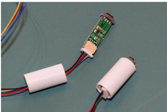
With the detector wires connected, insert the detector into the tube. Orient the connector of the detector toward the shorter strip inside of the tube.
