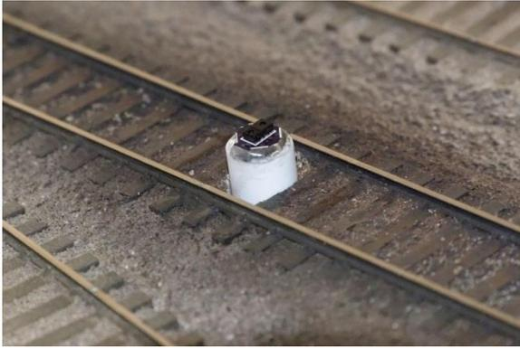
The inserted detector and holder are ready to align with the ends of the removed tie and to be pushed down into position.
