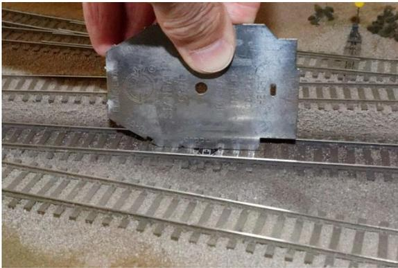
Use a straight edge to level the sensor head of the detector with the adjacent ties.
