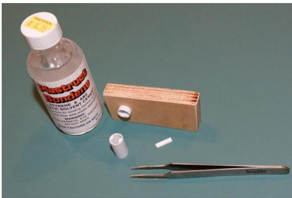
The styrene strips are glued to opposite sides of the interior of the tube.
