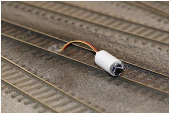
Remove the tie at the detector location, and drill a 3/8" hole between the adjoining ties. There's almost always just enough room for this.
