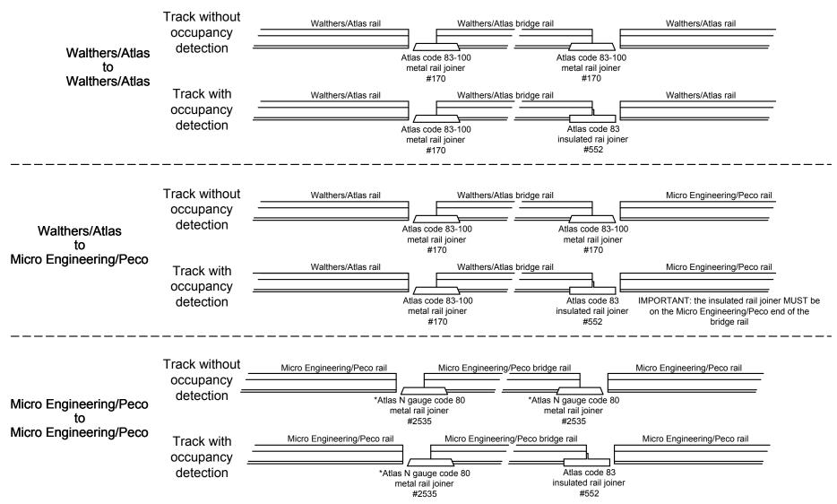
\*Micro Engineering metal rail joiner 26-083 may be used if prepared by running it onto a spare piece of rail before using.
